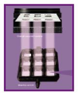
2. The CCD Camera is made up of a collection of light sensitive diodes which convert light into electrons to produce an electrical charge. The brighter the light that hits a single diode, the greater the electrical charge that will accumulate at that site.
