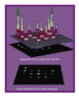
4. A validated biochip image is then produced, which undergoes image analysis for quantification of the signal output at each DTR.
